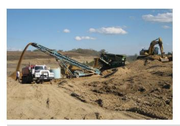
**Project Description:** As tonnage increases the trash shredder will be used for larger waste items, such as construction debris. Shredding this material will save air space prolonging the lifespan of the current landfill site.
